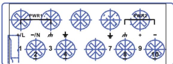
**STEP 1:** Insert the dual set positive/negative DC wires into PWR1 and PWR2 terminals (+ → pins 1, 9; - → pins 2, 10).
