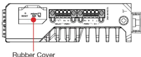
Insert the microSD card into the slot. Make sure you insert the card in the correct direction. There is an image above the slot indicating the direction that the microSD card should be inserted.
