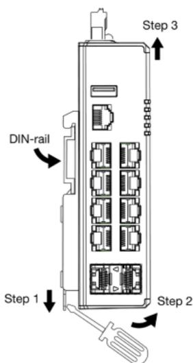
**NOTE** Screws that are used to fix the DIN-rail kit on the TSN-G5000 Series should be securely fastened before mounting on the mounting rail. Please make sure that if you remove the DIN-rail kit, it must be securely fastened when it is reattached.
