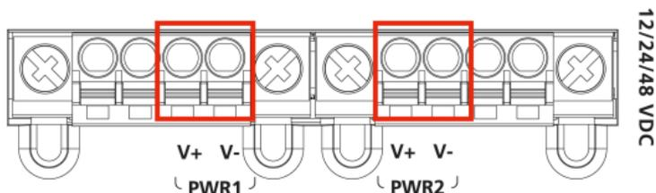
Take the following steps to wire the redundant power inputs:
