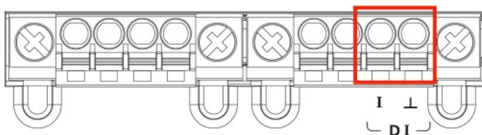
**Step 1**—Insert the negative (ground)/positive DI wires into the respective  $\perp$ /I terminals.
