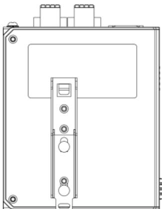
**Step 2**—Insert the upper lip of the DIN-rail kit into the mounting rail.
