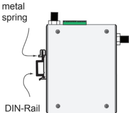
To remove the AWK-1131A from the DIN-Rail, simply reverse Steps 1 and 2.
