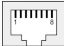
**NOTE** The pin numbers for both 8-pin and 10-pin RJ45 connectors (and ports) are typically not labeled on the connector (or port). Refer to the Pinout diagram above to see how RJ45 pins are numbered.
