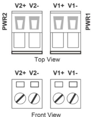
**STEP 1:** Insert the negative/positive DC wires into the V+/V- terminals, respectively.
