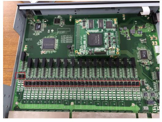
In some critical environments, you may need to add termination resistors to prevent the reflection of serial signals. When using termination resistors, it is important to set the pull high/low resistors correctly so that the electrical signal is not corrupted. The DA-660A uses jumper settings to set the termination resistors and pull high/low resistor values for each serial port.
