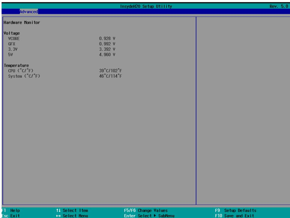
Note that the voltage values vary depending on the model. The temperature readings shown on the screen are within  $\pm 5\%$  of the actual readings. However, the temperature readings are only valid when the ambient temperature is above 0°C.
