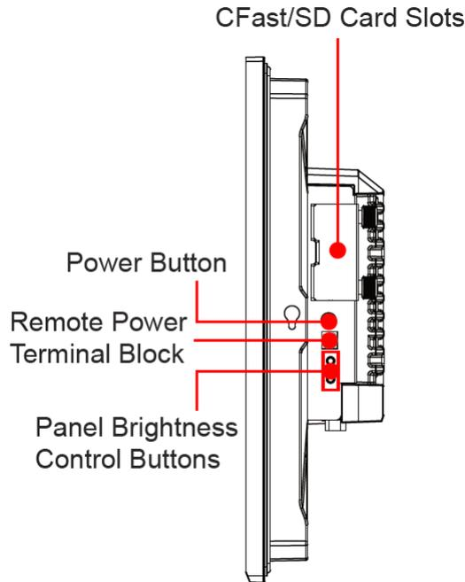
The usage of the display-control buttons is described in the following table:
