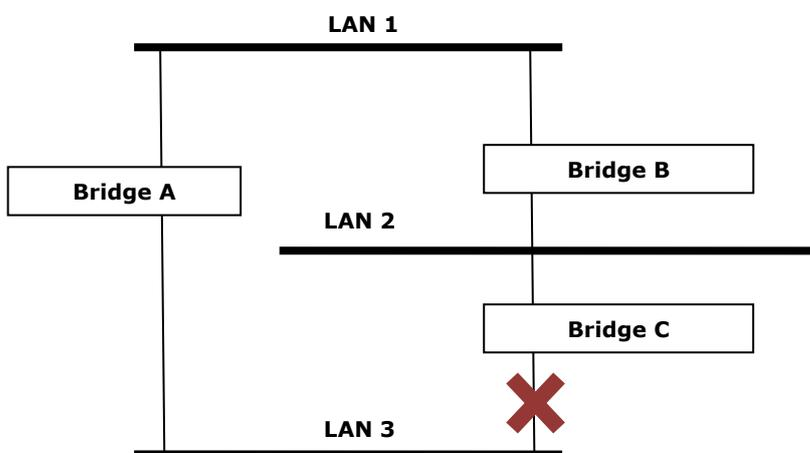
STP will determine which path between each bridged segment is the most efficient and then assign a specific reference point on the network. When the most efficient path has been identified, the other paths are blocked. In the above three figures, STP first determined that the path through Bridge C was the most efficient, and as a result, blocked the path through Bridge B. After the failure of Bridge C, STP reevaluated the situation and opened the path through Bridge B.
