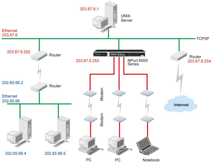
In this example, dial-in users can make requests to Intranet hosts **202.65.66.4** or **202.65.66.5**, which are on network **202.65.66.xxx** (located outside network **203.67.6.xxx**). You will need to add a route entry for the next-hop router, **203.67.6.252** that delivers requests to network **202.65.66.xxx**. The metric hop in this case is 2 route hops.
