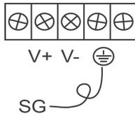
The Shielded Ground (sometimes called Protected Ground) contact is the second contact from the right of the 5-pin power terminal block connector located on the rear panel of the NPort 6600 VDC. Connect the SG wire to the earth ground.
