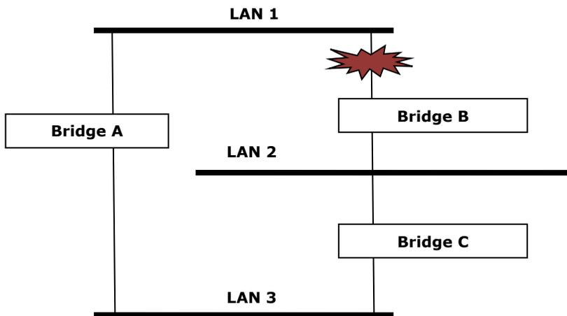
What happens if a link failure is detected? As shown in next figure, the STP process reconfigures the network so that traffic from LAN segment 2 flows through Bridge B.
