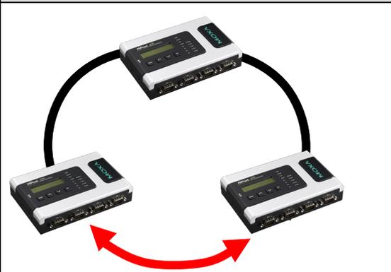
If there are  $2N+1$  NPort 6000 units (an odd number) in the Turbo Ring, with NPort 6000 units and segments labeled counterclockwise, then segment  $N+1$  will serve as the backup path.
