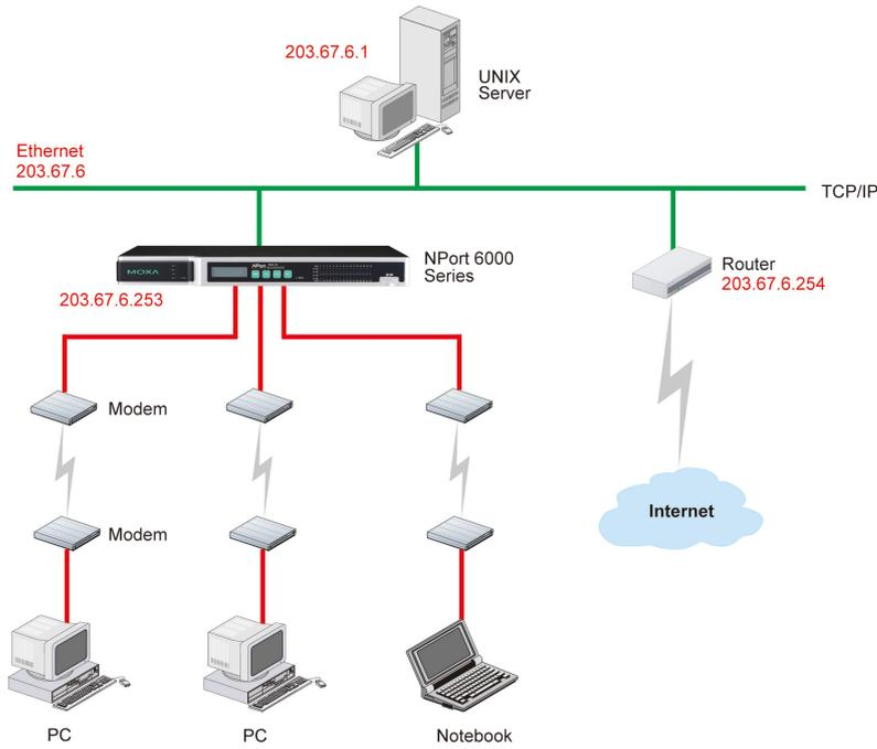
In this example, the Notebook PC dials into the NPort 6000 to request a connection to the Internet host at **210.48.96.9**, which is not on the local network **203.67.6.xxx**. This causes the NPort 6000 to act as a router and send the datagram to the default next-hop router, **203.67.6.254**. In this case, we should add the gateway IP address of **203.67.6.254** to the routing table to handle hops to **210.48.96.9**.
