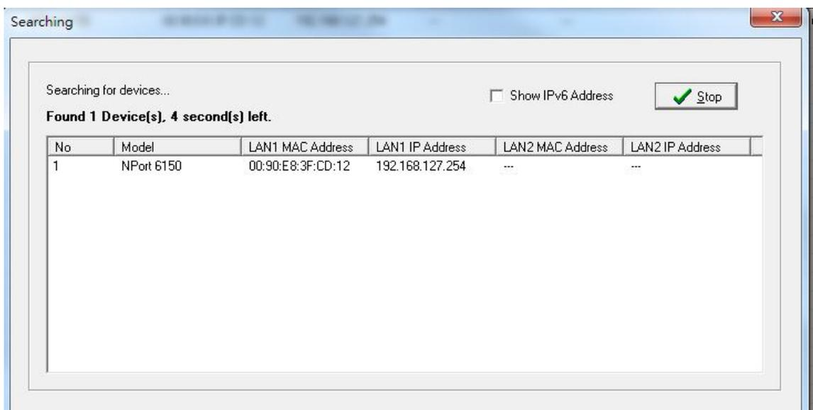
2. When the search is complete, all NPort 6000 servers that were located will be displayed in the DSU window. Select the device you wish to access and press the **UnLock** button to input the username and password for the device. (The username is mandatory for NPort 6000 series installed with firmware v1.14 and above.)
