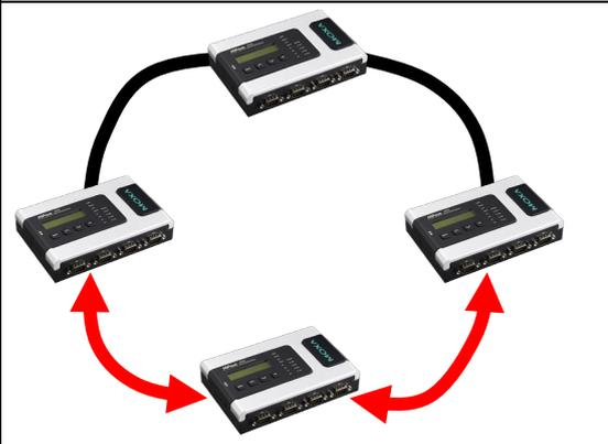
If there are  $2N$  NPort 6000 units (an even number) in the Turbo Ring, then the backup segment is one of the two segments connected to the  $(N+1)$ st NPort 6000 (i.e., the NPort 6000 unit directly opposite the master).
