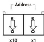
Before communicating, you must assign a slave ID to the PROFIBUS slave. If you would like to assign an address between 0 to 99, you need to change the rotary switch to the desired address. If you would like to assign an address which is over 99, you must set it via web console.
