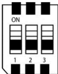
On the MGate 5118's left side panel, you will find DIP switches to adjust each CAN port or serial port's pull-high resistor, pull-low resistor, and terminator.
