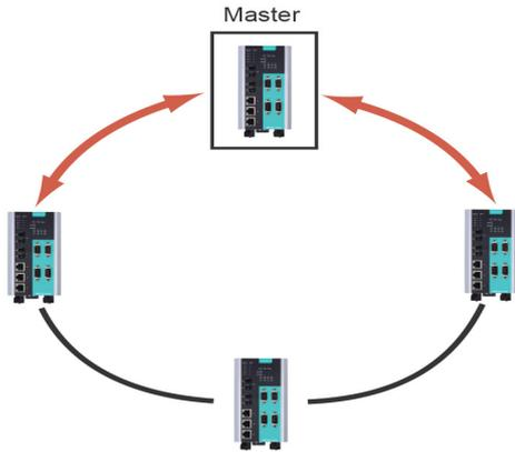
For a "Turbo Ring V2" ring, the backup segment is the segment connected to the second redundant port on the master.
