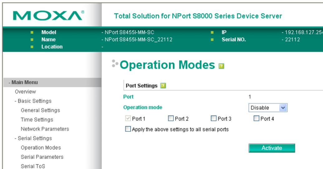
When Operation mode is set to Disabled, that particular port will be disabled. Check the **Apply the above settings to all serial ports** to apply this setting to the other port.
