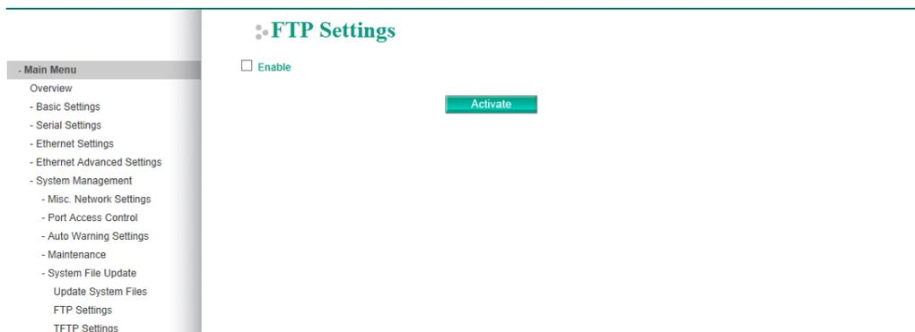
The NPort S9000 can be a FTP server to save configuration file or log files on it. You may enable it by checking the checkbox **Enable** and then click **Activate**.
