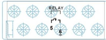
**FAULT:** The relay contact of the 10-pin terminal block connector is used to detect user-configured events. The two wires attached to the RELAY contacts form an open circuit when a user-configured event is triggered. If a user-configured event does not occur, the RELAY circuit will be closed.
