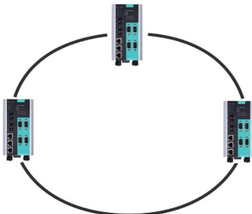
1. For each NPort S9000 in the ring, select any two ports as the redundant ports.
