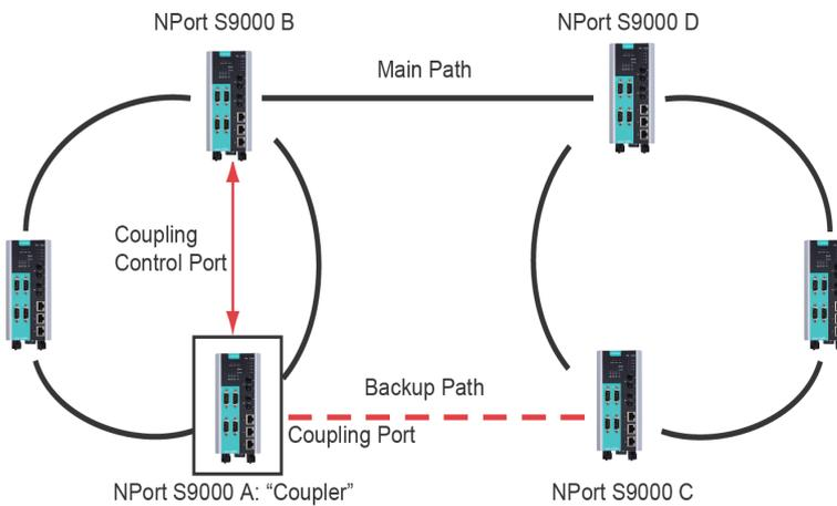
To configure the Ring Coupling function for a "Turbo Ring" ring, select two NPort S9000 devices (e.g., Device A and B in the above figure) in the ring, and another two NPort S9000 devices in the adjacent ring (e.g., Device C and D).
