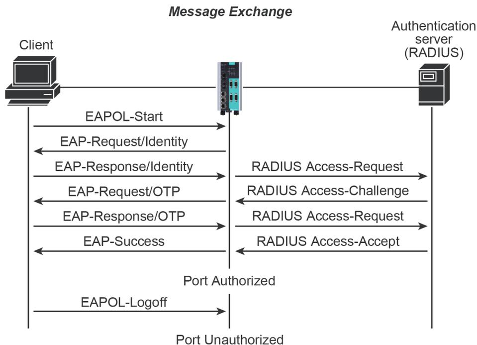
1. When the supplicant receives an "EAP Request/Identity" frame, it sends an "EAP Response/Identity" frame with its username back to the authenticator.
