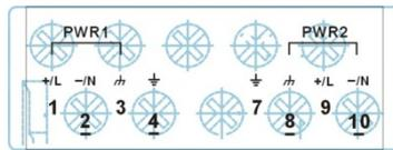
STEP 1: Insert the dual set positive/negative DC wires into PWR1 and PWR2 terminals (+ → pins 1, 9; - → pins 2, 10). Or insert the L/N AC wires into PWR1 and PWR2 terminals (L → pin 1, 9; N → pin 2,10)
