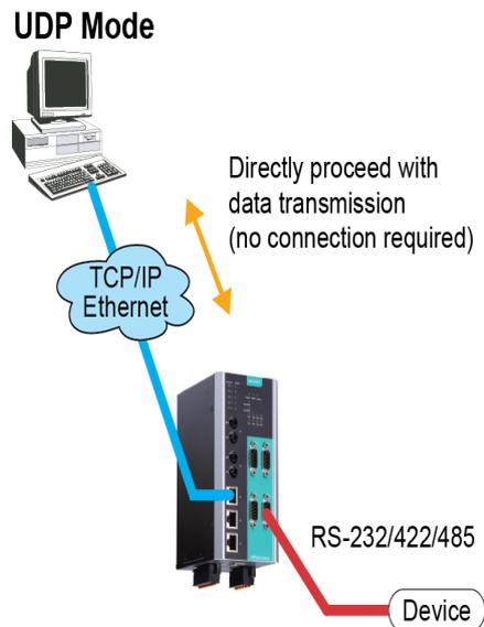
The NPort S9000 series also can be a gateway to support three kinds of communication protocols: DNP3, DNP3 Raw Socket and Modbus. For the NPort S9000 series, each serial port can be set to different protocols.
