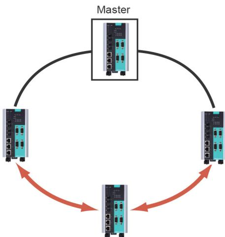
If there are  $2N$  NPort S9000 (an even number) in the “Turbo Ring” ring, then the backup segment is one of the two segments connected to the  $(N+1)$  NPort S9000 (i.e., the NPort S9000 unit directly opposite the master).
