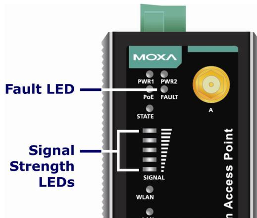
The following table summarizes how to read the device's wireless settings from the LED displays. More information is available in Chapter 3 in the "Basic WLAN Setup" section.
