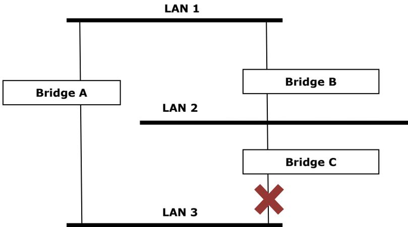
STP will examine each bridged segment determine which path is most efficient, and then assign a specific reference point on the network. When the most efficient path has been identified, the other paths are blocked. In the previous 3 figures, STP first determined that the path through bridge C was the most efficient, and as a result, blocked the path through bridge B. After the failure of bridge C, STP re-evaluated the situation and opened the path through Bridge B.
