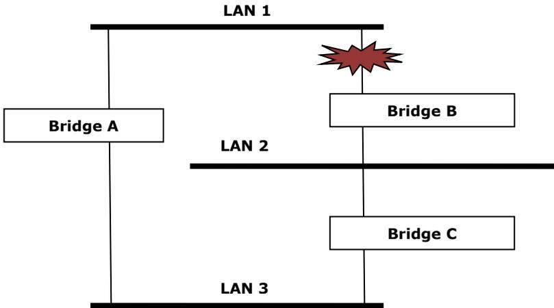
What happens if a link failure is detected? As shown in the next figure, the STP process reconfigures the network so that traffic from LAN segment 2 flows through bridge B.
